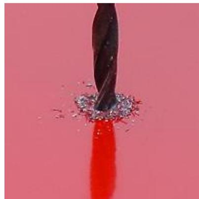
Please note it's important to drill at low speed, with a maximum of 500 rounds per minute. Do not apply too much pressure during drilling.
